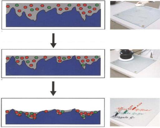
Fig8: the functional principle of a colored protective coating retrofitted to a glass surface:
