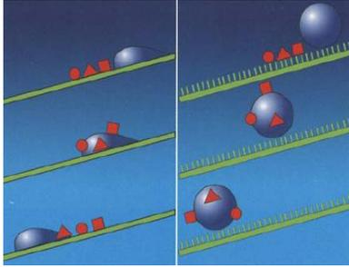
Fig12: The diagrams show clearly the difference between conventional surfaces and the Lotus-Effect.<sup>1</sup>
