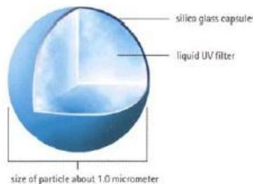
Fig16: Silica glass capsules are used in nanoporous anti-reflective coatings with a thickness of 150 nm that are also able to reflect the invisible spectrum of light.<sup>4</sup>
