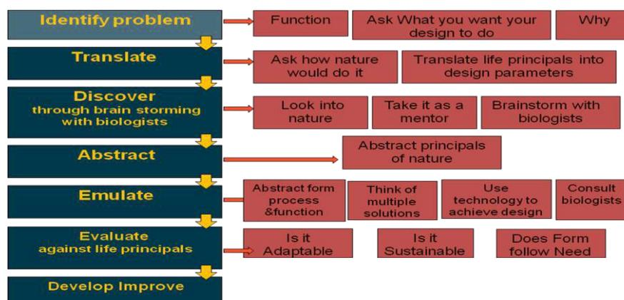
Fig.18 Design methodology diagram based on Benyus's Challenge to Biology Design Spiral.
