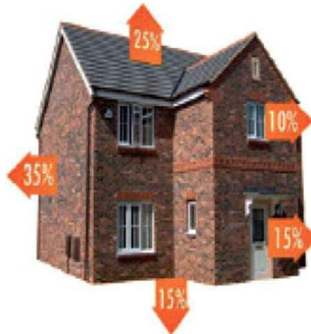
**Figure 8: Main building elements and proportions of heat loss due to lack of efficient insulation (Power, 2008)**
