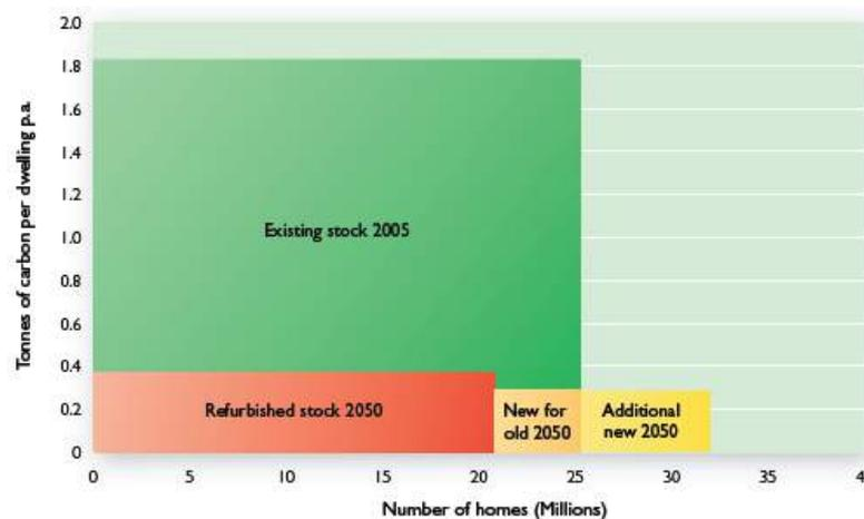
Figure 7: CO<sub>2</sub> emissions from refurbished and new-build housing (Killip, 2008)
