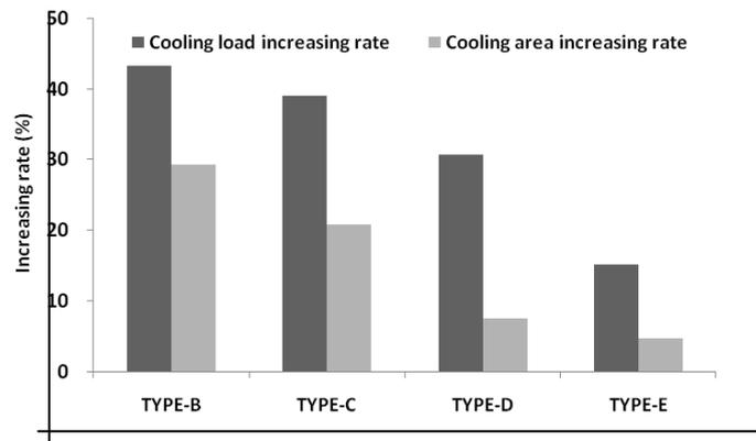
Fig.4 The bias of the increasing rate of cooling load and cooling area from type-A
