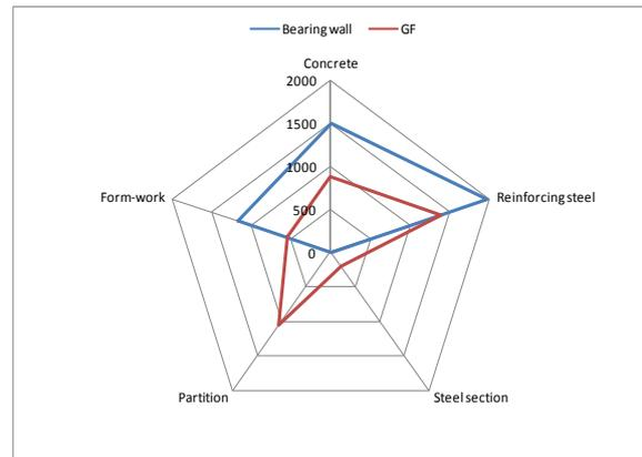
Fig.5 Energy consumption per unit area for each structural type
