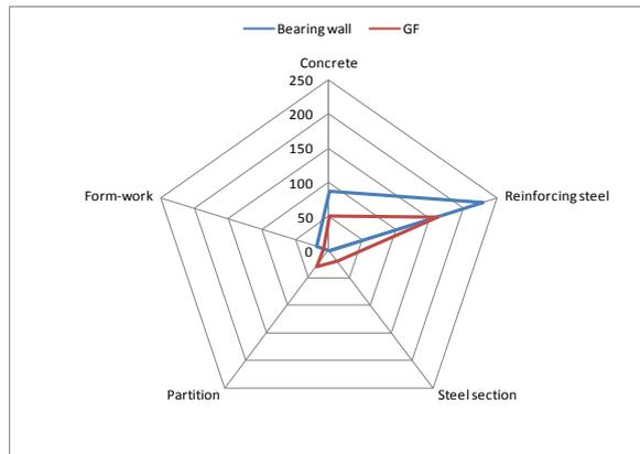
Fig.4 CO<sub>2</sub> emission per unit area for each structural type
