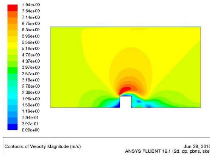
**Fig.5 Velocity Contours of velocity magnitudes for coarse fine mesh**
