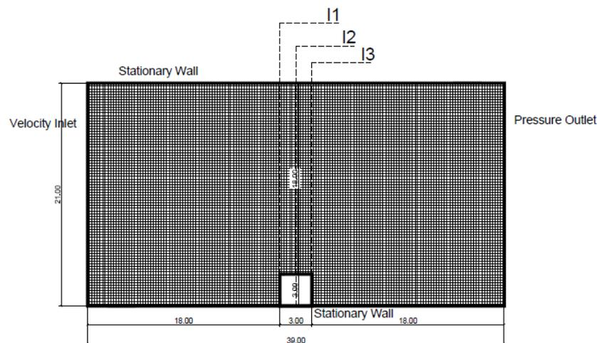
**Fig.2 Domain geometry and specifications**
