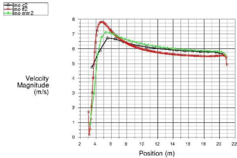
Fig.7 Velocity magnitude plot along line l2 for coarse (c1), medium (mm1) and fine (ff1) meshes
