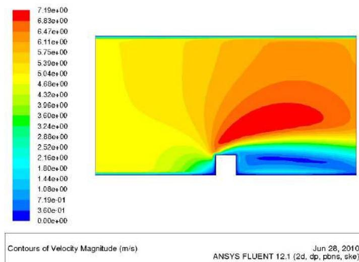
**Fig.4 Velocity Contours of velocity magnitudes for medium mesh**
