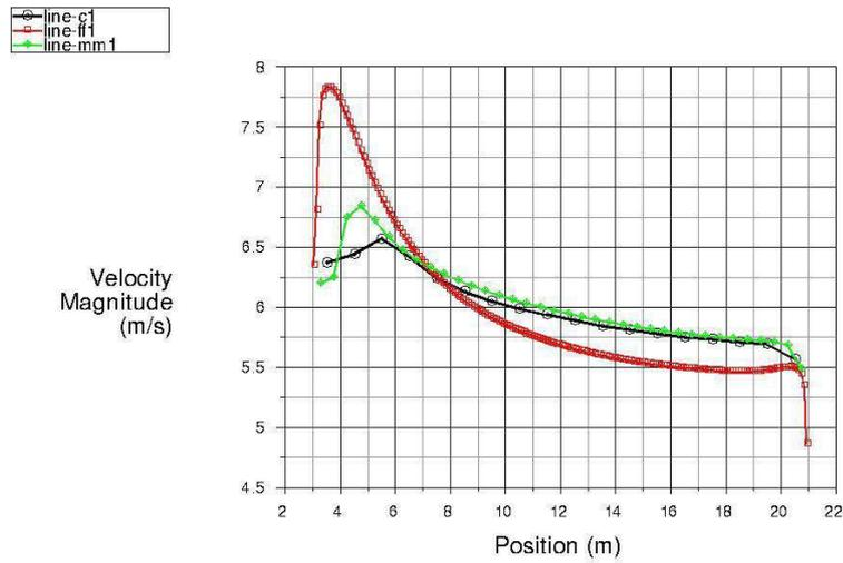
Fig.6 Velocity magnitude plot along line l1 for coarse (c1), medium (mm1) and fine (ff1) meshes
