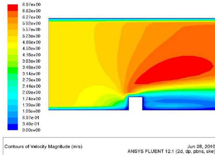
**Fig.3 Velocity Contours of velocity magnitudes for coarse mesh**
