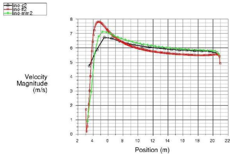
Fig.8 Velocity magnitude plot along line l3 for coarse (c1), medium (mm1) and fine (ff1) meshes
