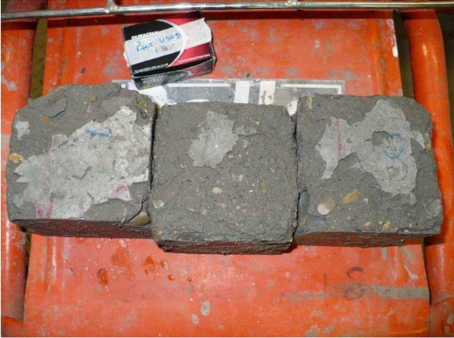
**Plate 1. Plain concrete cubes at 50 freeze/thaw cycles**
