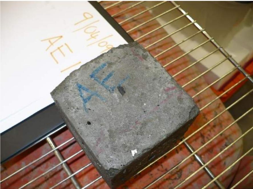
**Plate 2. Air Entrained sample at 50 freeze/thaw cycles**
