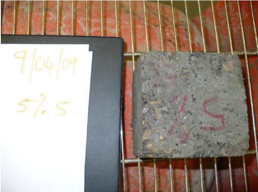
**Plate 3. 5% Rubber sample at 50 freeze/thaw cycles.**
