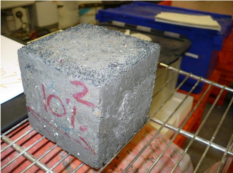
**Plate 4. 10% Rubber sample at 50 freeze/thaw cycles**
