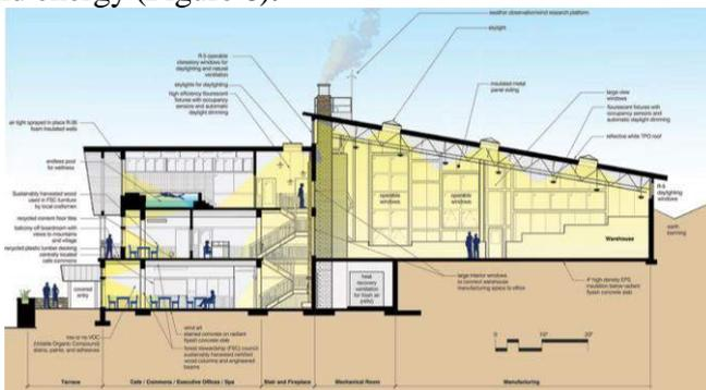
**Fig.6 Building Cross Section Showing Skylights. (William Maclay Architects & Planners, 2008).**
