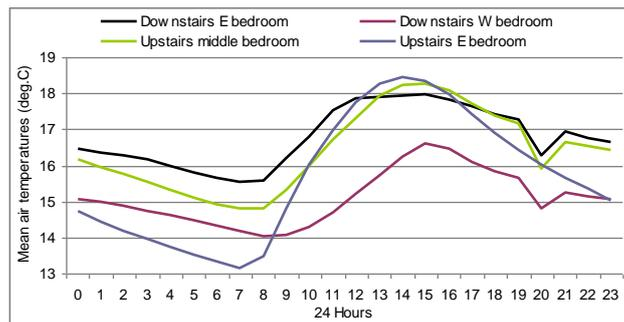
Fig.7 Mean air temperatures of upstairs and downstairs bedrooms
