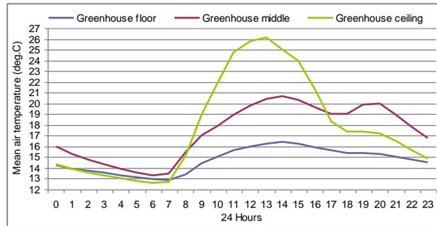
Fig.6 Mean air temperatures of the courtyard space of the 'wind-rain' house
