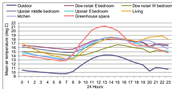
**Fig.4 Hourly mean temperatures during the winter months of the 'wind-rain' house**
