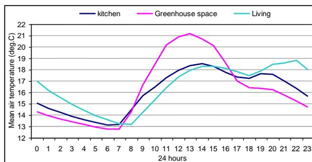
**Fig.5 Mean air temperatures of the courtyard space and downstairs kitchen and living**
