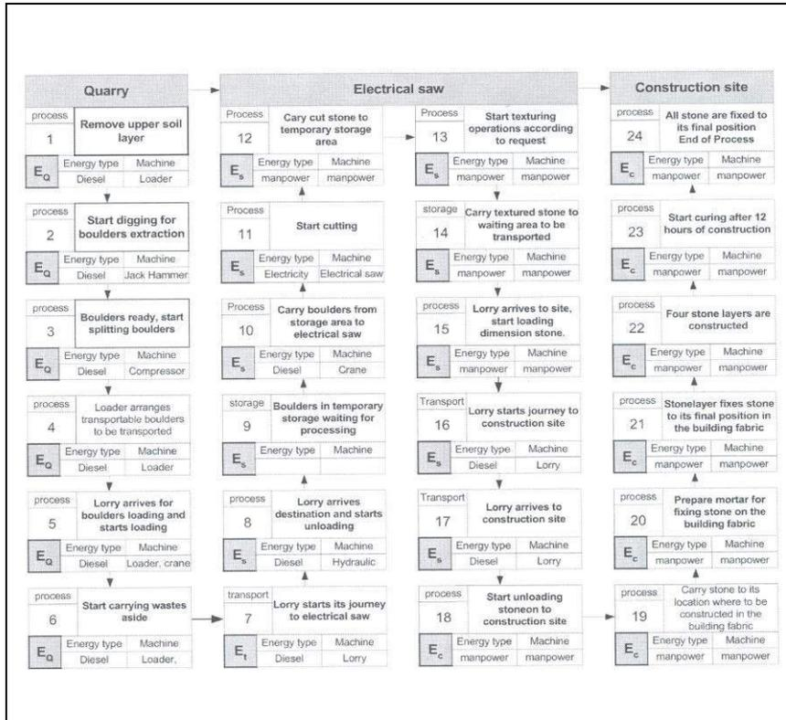
Fig. 2: an example of modern building materials, dimensioned stone high energy consumption, low recycling possibilities, and high emissions to the environment. Shown the process chart for manufacturing. (Source: Alshboul & Alzoubi, 2008).
